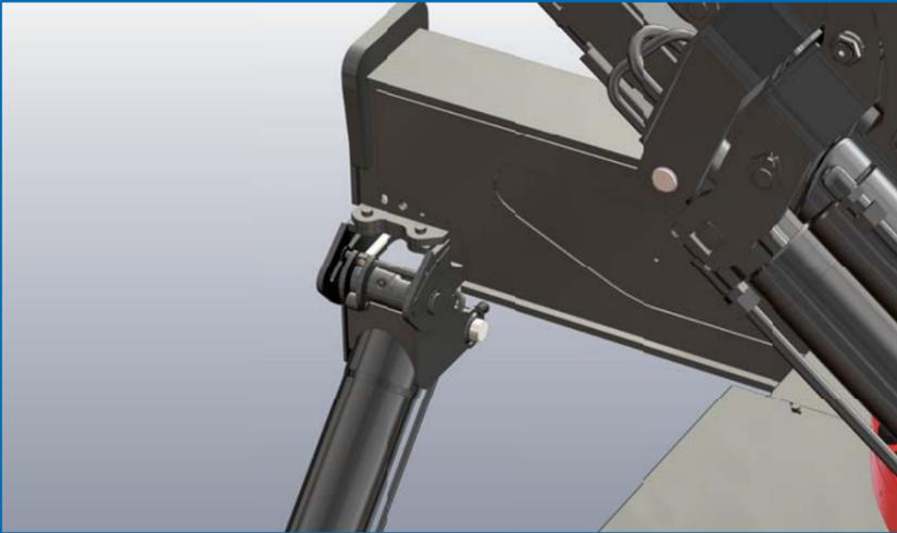
A distribution valve on the base of the crane ensures proportional oil distribution and protection against excess pressure, so that the speed remains even. At the same time, all the stabilizer functions can be run simultaneously for faster operation.
