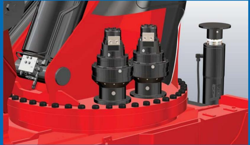
The new 2-gear slewing system makes operation even smoother and more stable. The gears are protected by a smart new cover, which you can easily take off and put on again if you have to take over control in an emergency.
