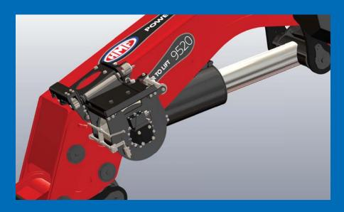
Now it is even easier to work with a hoist. The wire rope runs in automatically when you fold up the crane.
