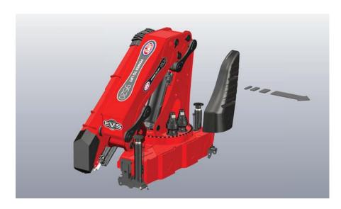
The shield is easy to lift off in one move.
